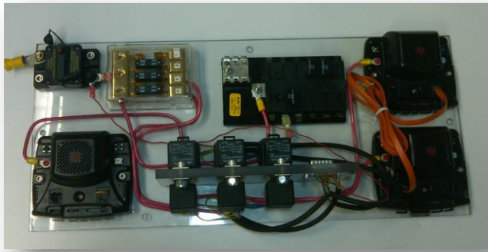
Figure 2: Final Power Board Design
